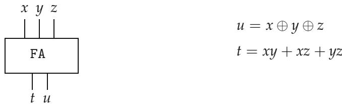
Figure 2.4 A full-adder (FA) cell. From three bits x, y, and z , it computes two bits t and u such that x + y + z = 2t + u .
